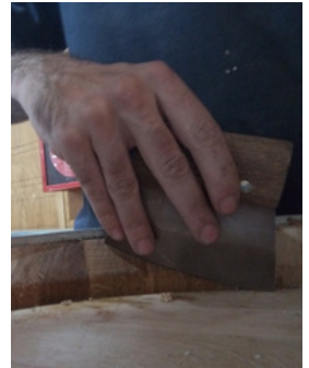
Scrape off the excess paraffin, remove the vacuum pump, and test the watertightness again.
