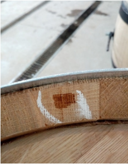
Locate the leak at the end of the stave.
