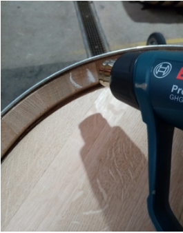
Heat the leak area
